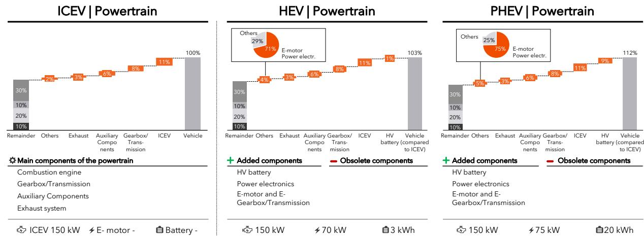
Costs for interior, exterior, chassis and E/E are assumed to be constant for all powertrains; 2 Costs for ICEV powertrain components are kept constant also for HEV and PHEV as power figures are similar
