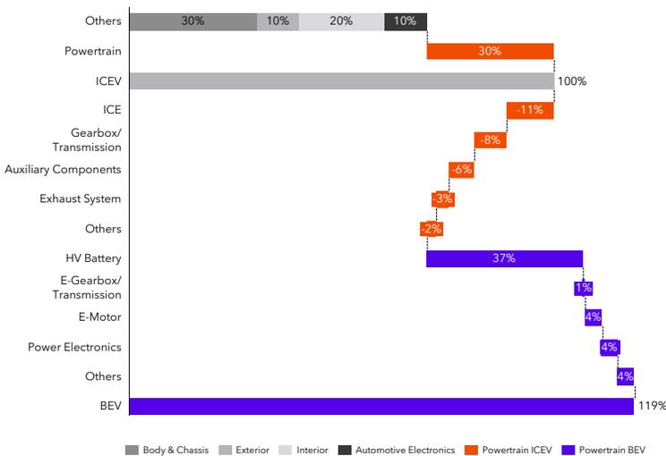
**Figure 22:** Component material cost share vs. the total vehicle cost (ICE vs. BEV)
