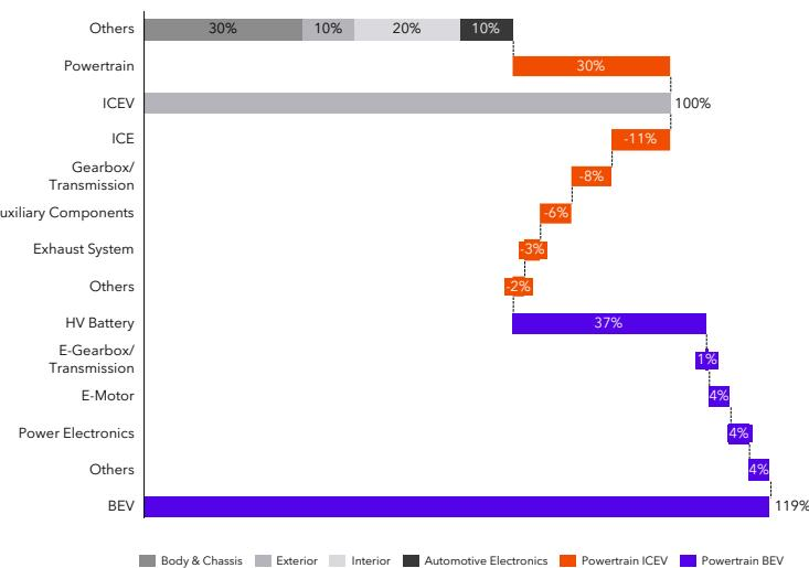
Figure 22: Component material cost share vs. the total vehicle cost (ICE vs. BEV)
