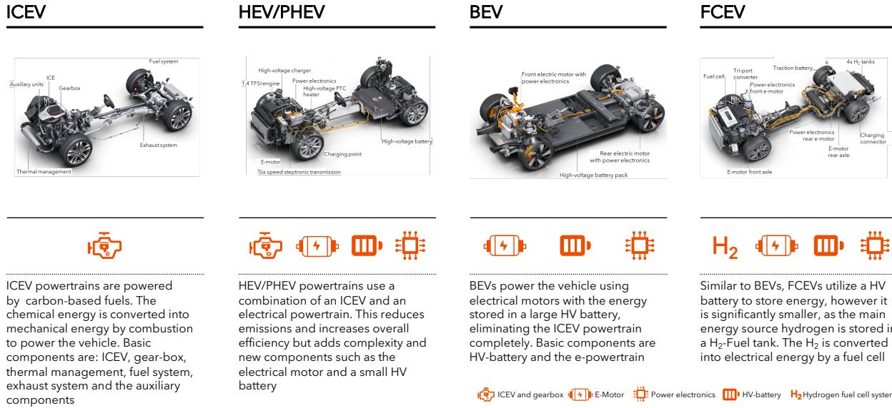
is more complex than that of an ICEV because it has both an ICE and electric powertrain.
